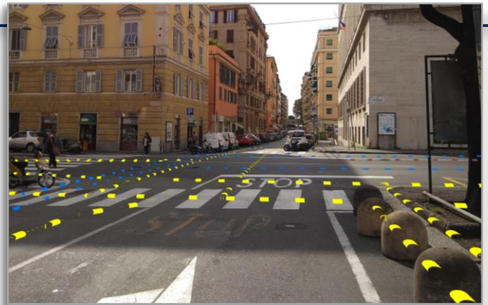
Augmented underground networks in Genoa, Italy
